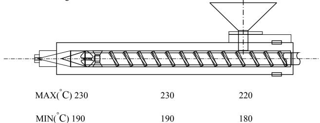
C. Mold Temperature  $30 \sim 70 \degree C$
