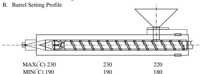
MIN(°C) 190 C. Mold Temperature 30~70 °C
